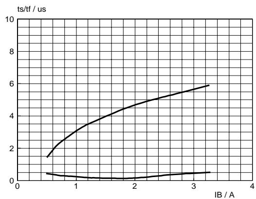
Fig.9. Typical collector storage and fall time.
