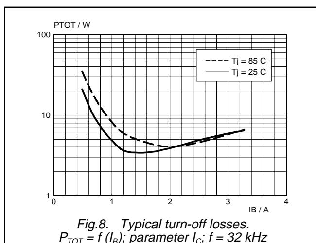
Fig.8. Typical turn-off losses.
