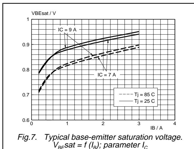
Fig.7. Typical base-emitter saturation voltage.
