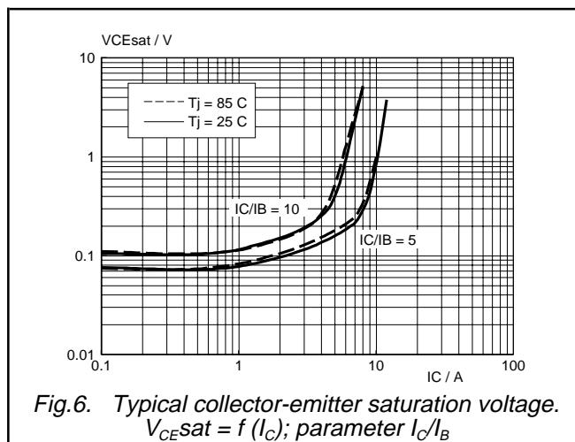
Fig.6. Typical collector-emitter saturation voltage.
