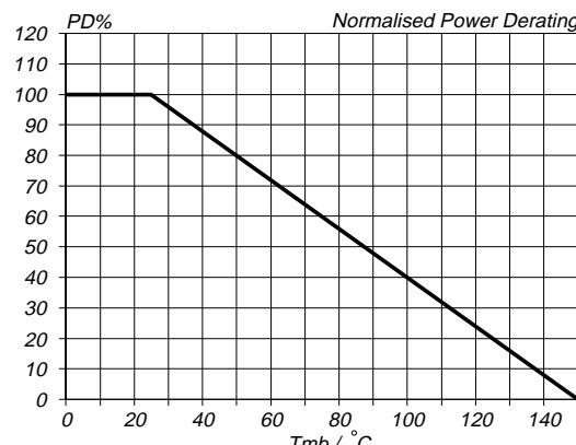
Fig.10. Normalised power dissipation.
