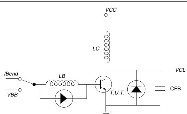
Fig.12. Test Circuit RBSOA.  $V_{CC} = 150$  V;
