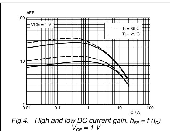
Fig.4. High and low DC current gain.  $h_{FE} = f(I_C)$
