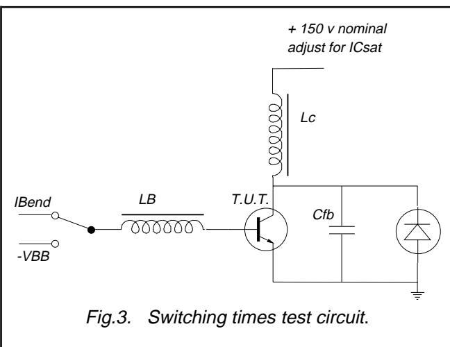
Fig.3. Switching times test circuit.
