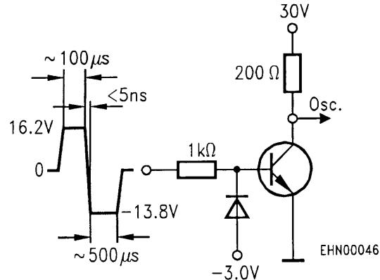
Oscillograph:  $R > 100 \text{ k}\Omega$
