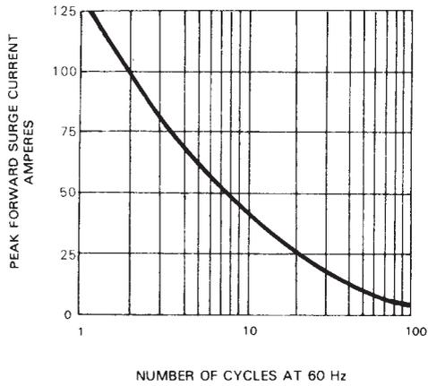
Fig. 2 – DERATING CURVE FOR OUTPUT RECTIFIED CURRENT
