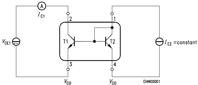
Note: Voltage drop at contacts:  $V_{CO} < \frac{2}{3} V_T = 16 \text{ mV}$
