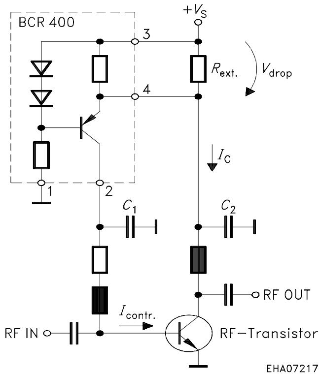
Be aware that BCR 400 stabilizes bias current of transistors in an active control loop.
