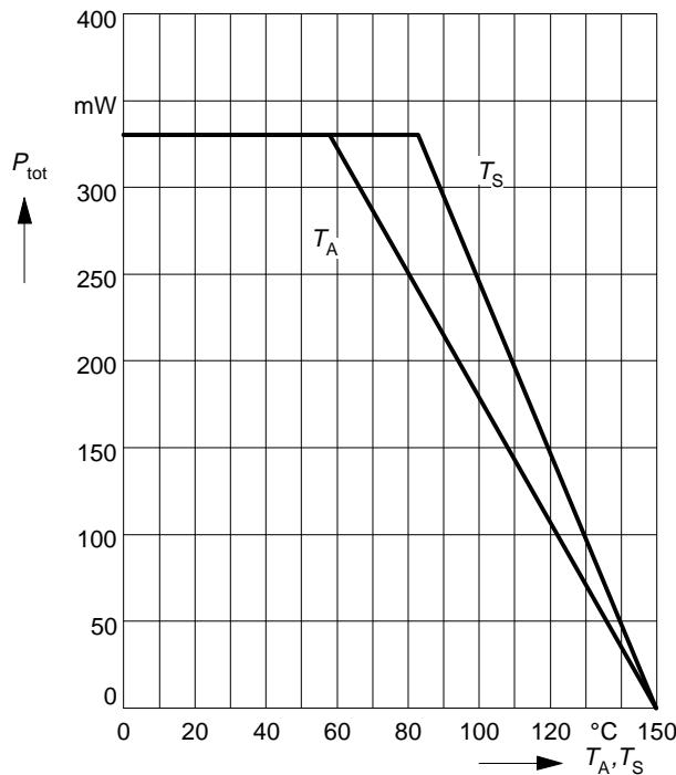
Note that up to  $T_S = 115^\circ\text{C}$  it is not possible to exceed  $P_{\text{tot}}$  respecting the maximum ratings of  $V_S$  and  $I_{\text{Contr.}}$ . The collector or drain current (respectively) of the stabilized RF transistor does not affect BCR 400 directly, as it provides just the base current.
