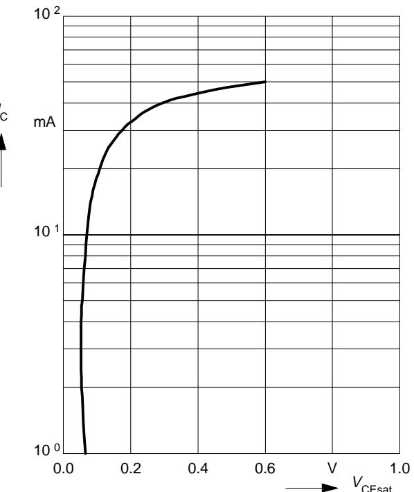
**Input off voltage**  $V_{i(off)} = f(I_C)$
