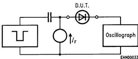
Pulse generator:  $t_p = 5\text{ }\mu\text{s}, D = 0.05$
