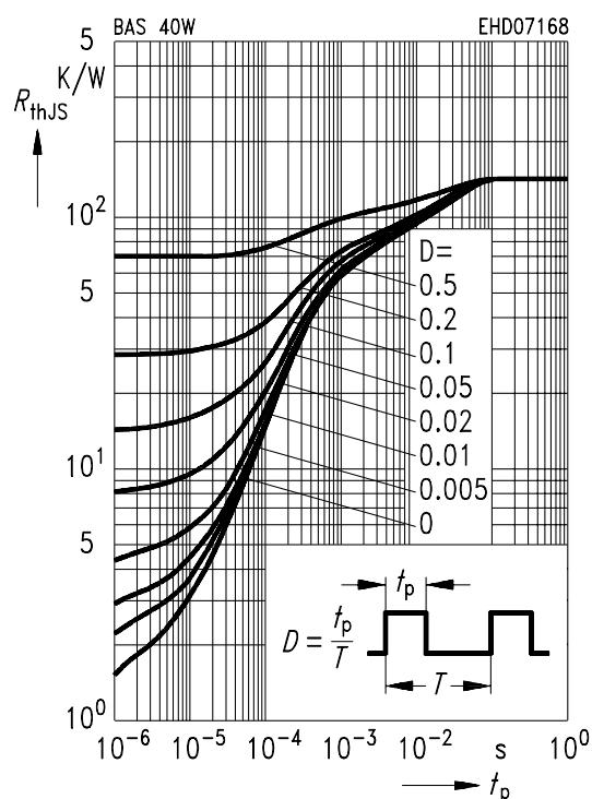
**Permissible Pulse load  $I_{Fmax}/I_{FDC} = f(t_p)$**
