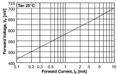
Figure 4. Forward Voltage vs Forward Current
