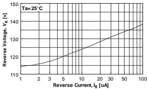
Figure 1. Reverse Voltage vs Reverse Current
