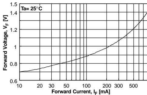
Figure 5. Forward Voltage vs Forward Current
