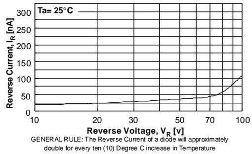
Figure 2. Reverse Current vs Reverse Voltage
