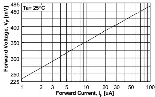
Figure 3. Forward Voltage vs Forward Current
