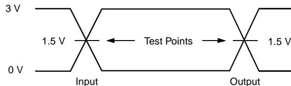
AC Testing for -70 devices: Inputs are driven at 3.0 V for a logic “1” and 0 V for a logic “0”. Input pulse rise and fall times are  $\leq 10$  ns.
