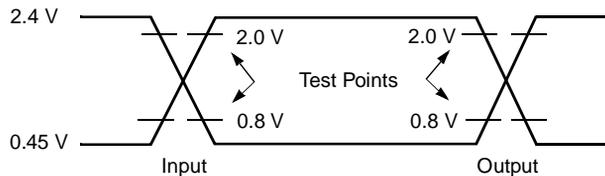
AC Testing (all speed options except -70): Inputs are driven at 2.4 V for a logic “1” and 0.45 V for a logic “0”. Input pulse rise and fall times are  $\leq 10$  ns.
