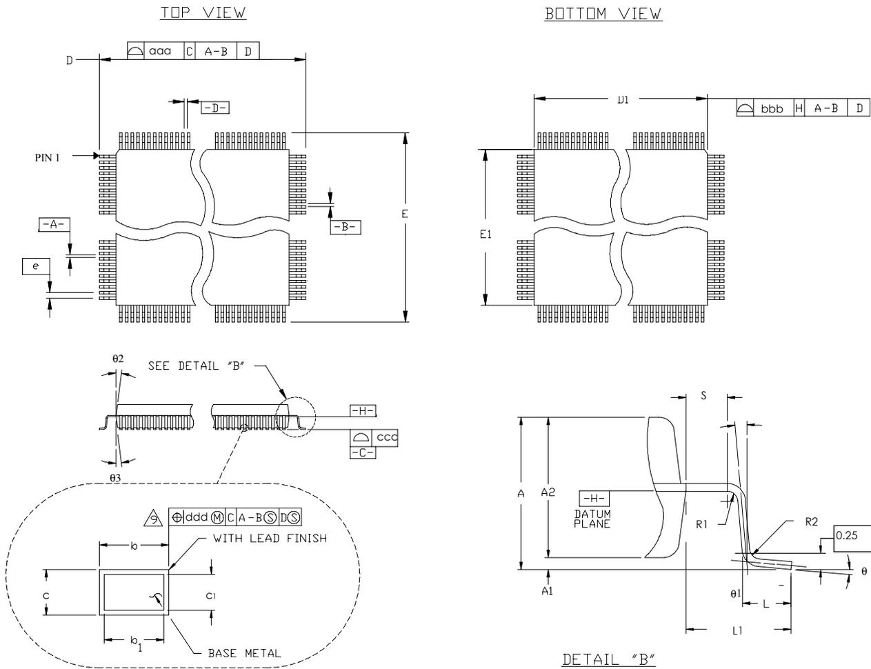
**Table 5.** Common Dimensions (mm) for 176-lead TQFP
