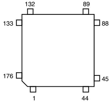
Figure 2. 176-ball BGA Pinout
