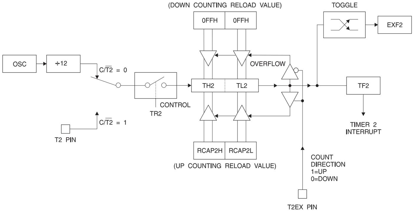
**Figure 4. Timer 2 in Baud Rate Generator Mode**
