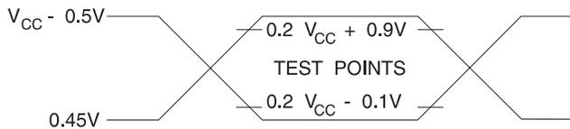
Notes: 1. AC Inputs during testing are driven at  $V_{CC} - 0.5V$  for a logic 1 and  $0.45V$  for a logic 0. Timing measurements are made at  $V_{IH}$  min. for a logic 1 and  $V_{IL}$  max. for a logic 0.
