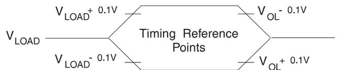
Notes: 1. For timing purposes, a port pin is no longer floating when a 100 mV change from load voltage occurs. A port pin begins to float when a 100 mV change from the loaded  $V_{OH}/V_{OL}$  level occurs.
