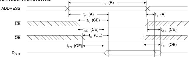
Notes: 1.  $\overline{\text{CE}}$  may be delayed up to t<sub>ACC</sub> - t<sub>CE</sub> after the address transition without impact on t<sub>ACC</sub>.
