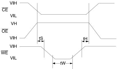
$$\begin{split} t_S &= t_H = 1 \; \mu sec \; (min.) \\ t_W &= 10 \; msec \; (min.) \\ V_H &= 12.0 \pm 0.5 V \end{split}$$
