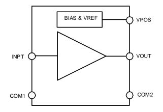
The noise figure is 3.9 dB at 900 MHz. The reverse isolation ( $s_{12}$ ) is - 33 dB at 900 MHz.
