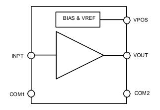
The noise figure is 5.1 dB at 900 MHz. The reverse isolation  $(s_{12})$  is - 36 dB at 900 MHz and -30 dB at 2.7 GHz.
