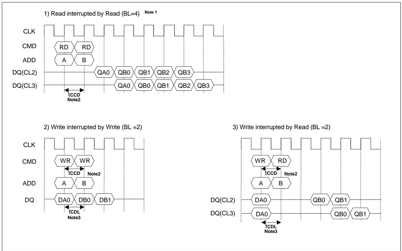
Note : 1. By "Interrupt", It is possible to stop burst read/write by external command before the end of burst.
