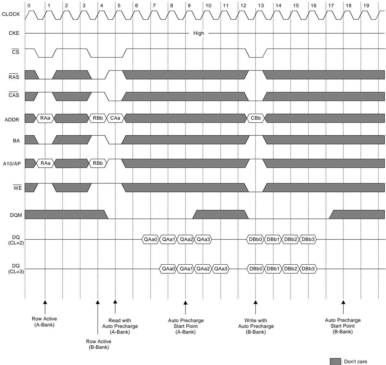
\*Note : tRCD should be controlled to meet minimum tRAS before internal precharge start.
