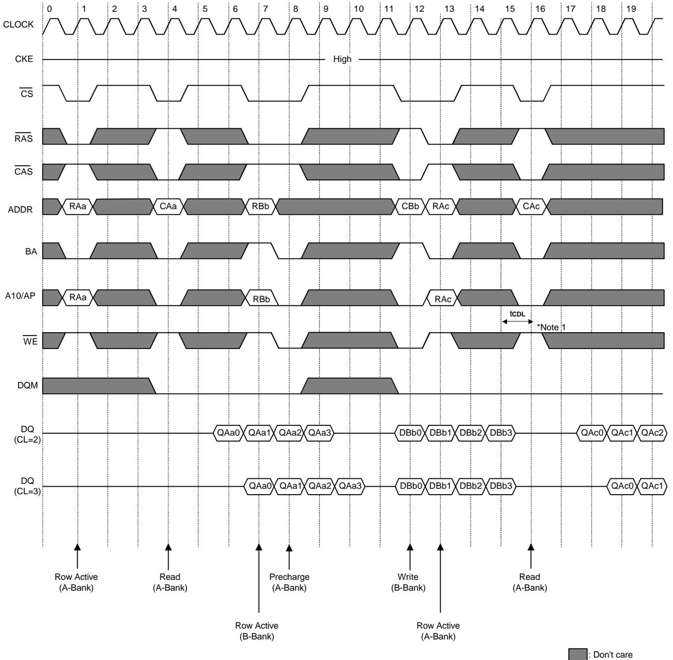
\* Note :  $t_{CDL}$  should be met to complete write.
