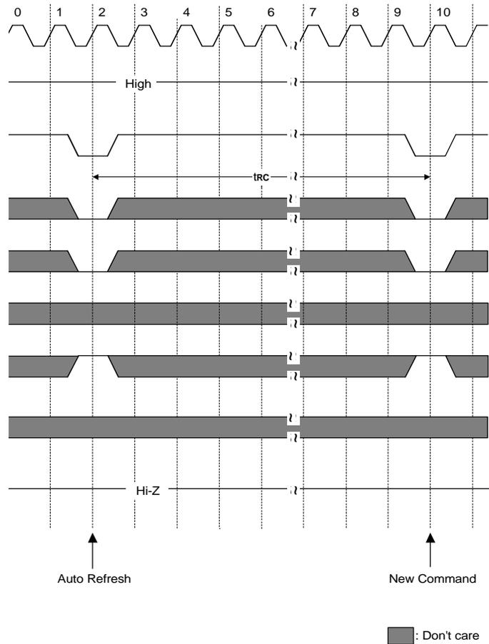
\* Both banks precharge should be completed before Mode Register Set cycle and auto refresh cycle.
