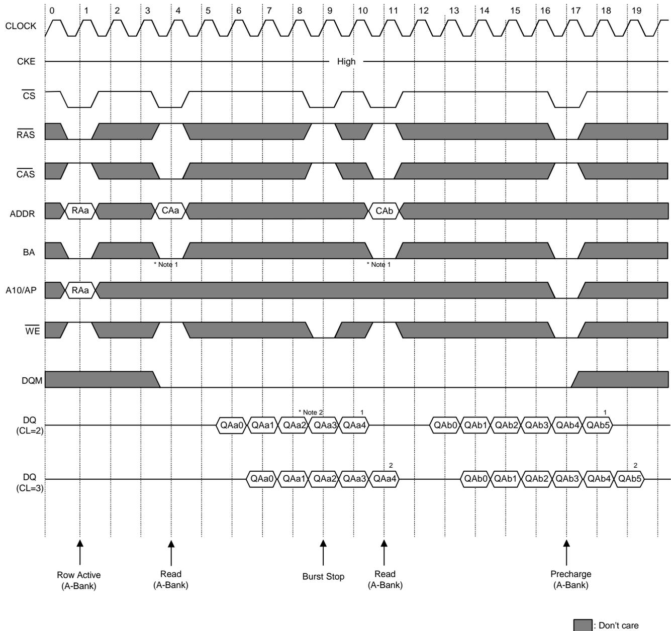
\* Note : 1. At full page mode, burst is wrap-around at the end of burst. So auto precharge is impossible.
