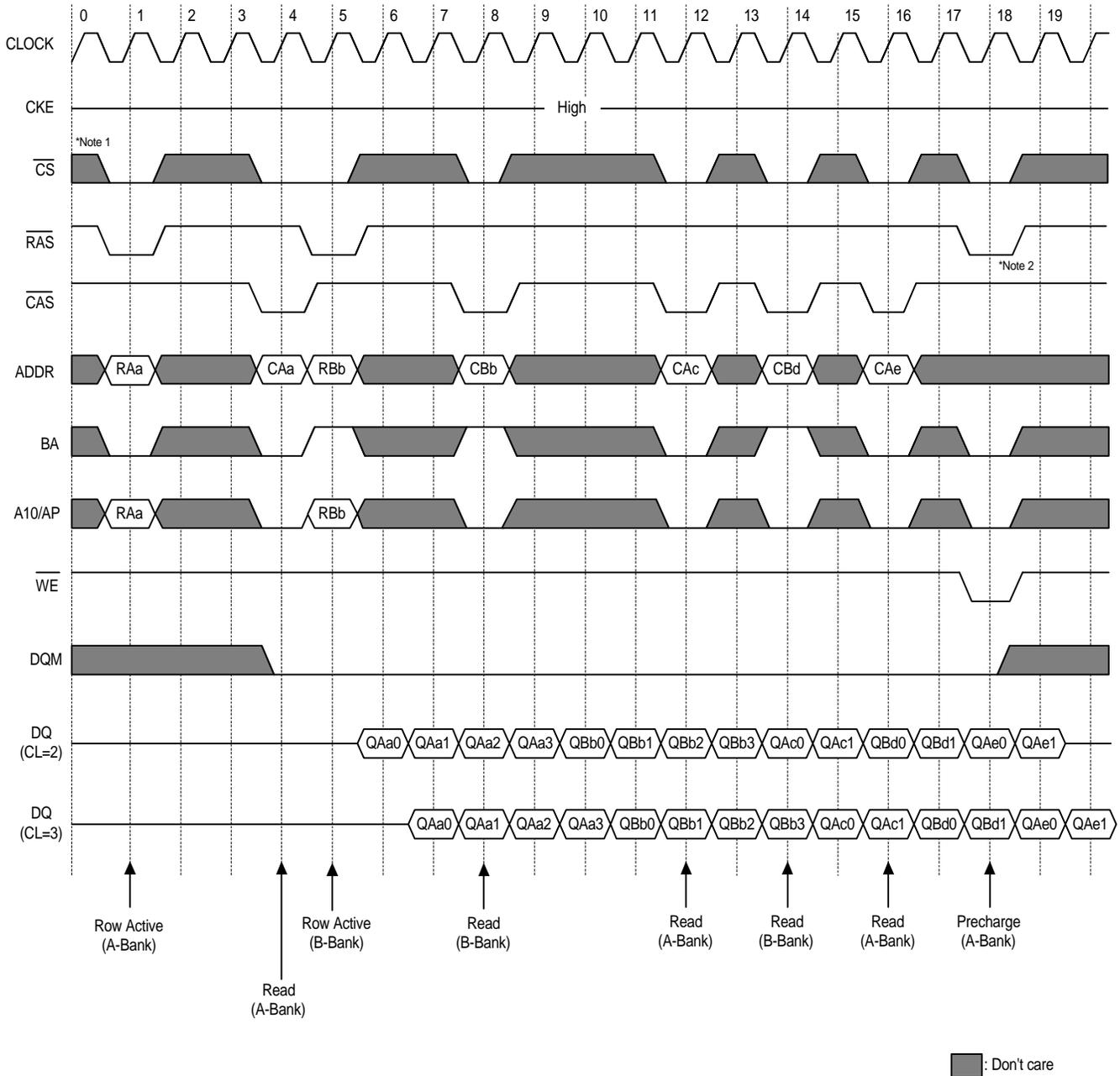
\* Note 1:  $\overline{CS}$  can be don't care when  $\overline{RAS}$ ,  $\overline{CAS}$  and  $\overline{WE}$  are high at the clock high going edge.
