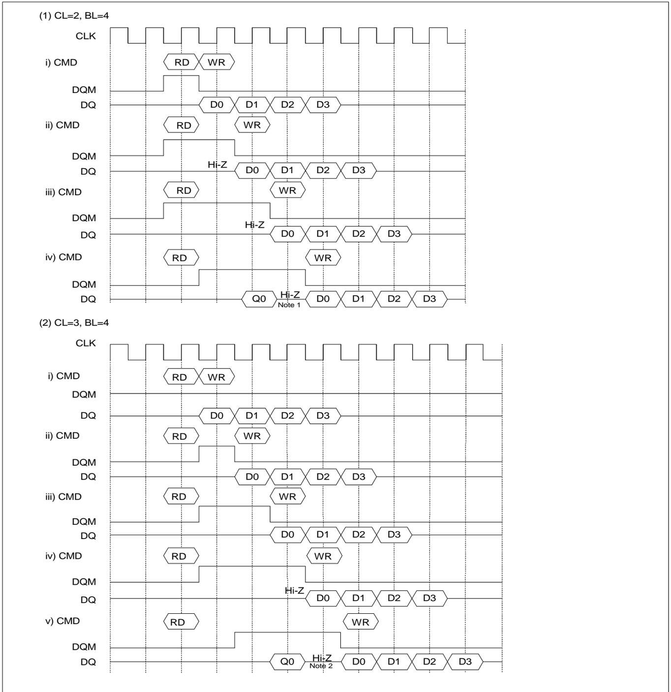
\* Note : 1. To prevent bus contention, there should be at least one gap between data in and data out.
