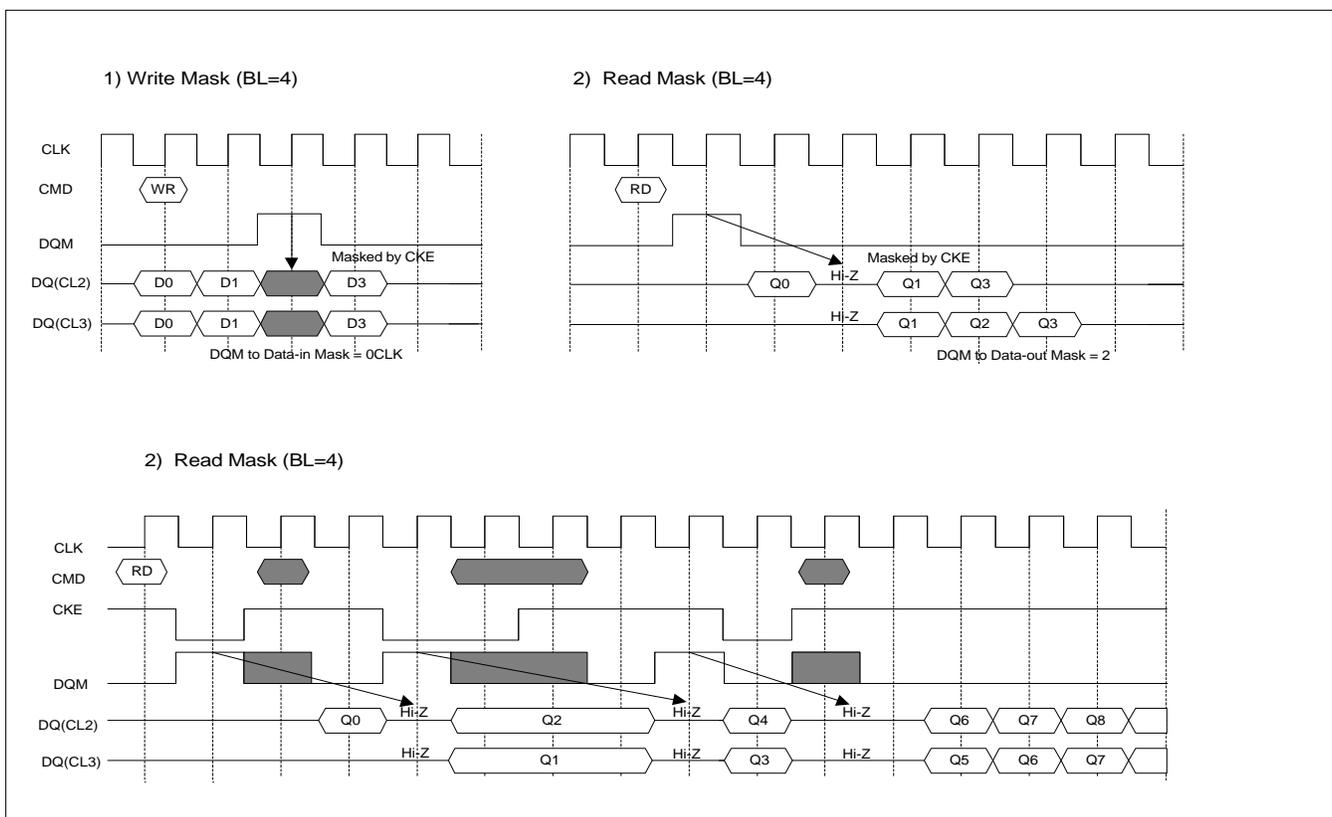
\* **Note** : 1. DQM makes data out Hi-Z after 2 clocks which should be masked by CKE "L".
