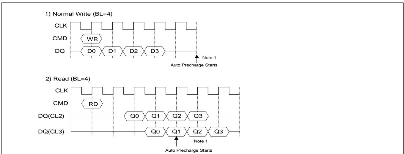
\* Note : 1. The row active command of the precharge bank can be issued after  $t_{RP}$  from this point.
