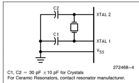
Figure 3. Oscillator Connections
