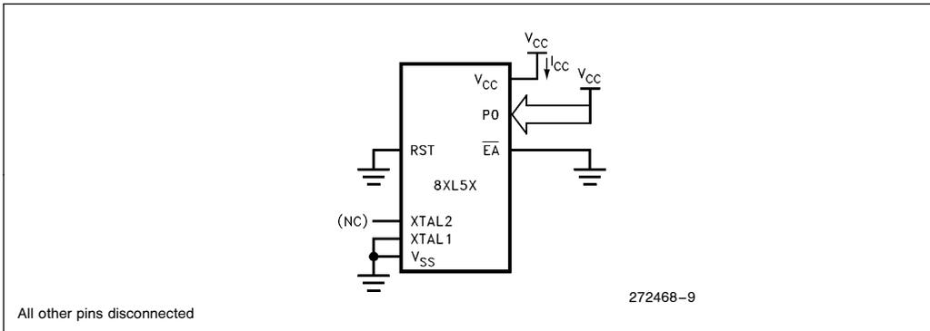
Figure 8.  $I_{CC}$  Test Condition, Power Down Mode.
