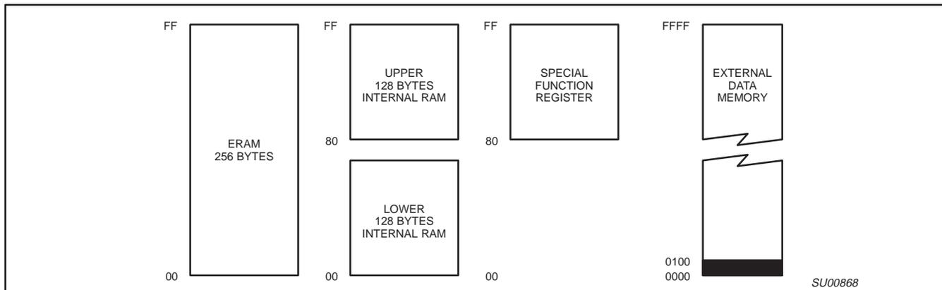
Figure 8. Internal and External Data Memory Address Space
