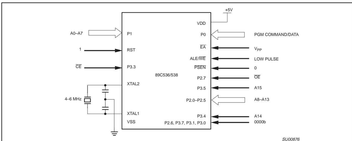
Figure 21. Erase/Programming/Verification
