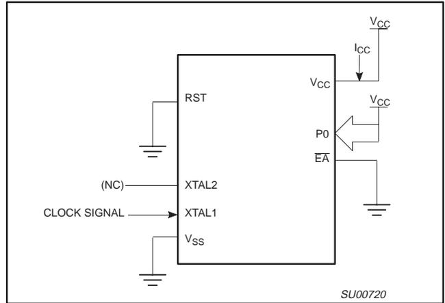
Figure 18.  $I_{CC}$  Test Condition, Idle Mode
