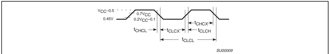
Figure 19. Clock Signal Waveform for  $I_{CC}$  Tests in Active and Idle Modes
