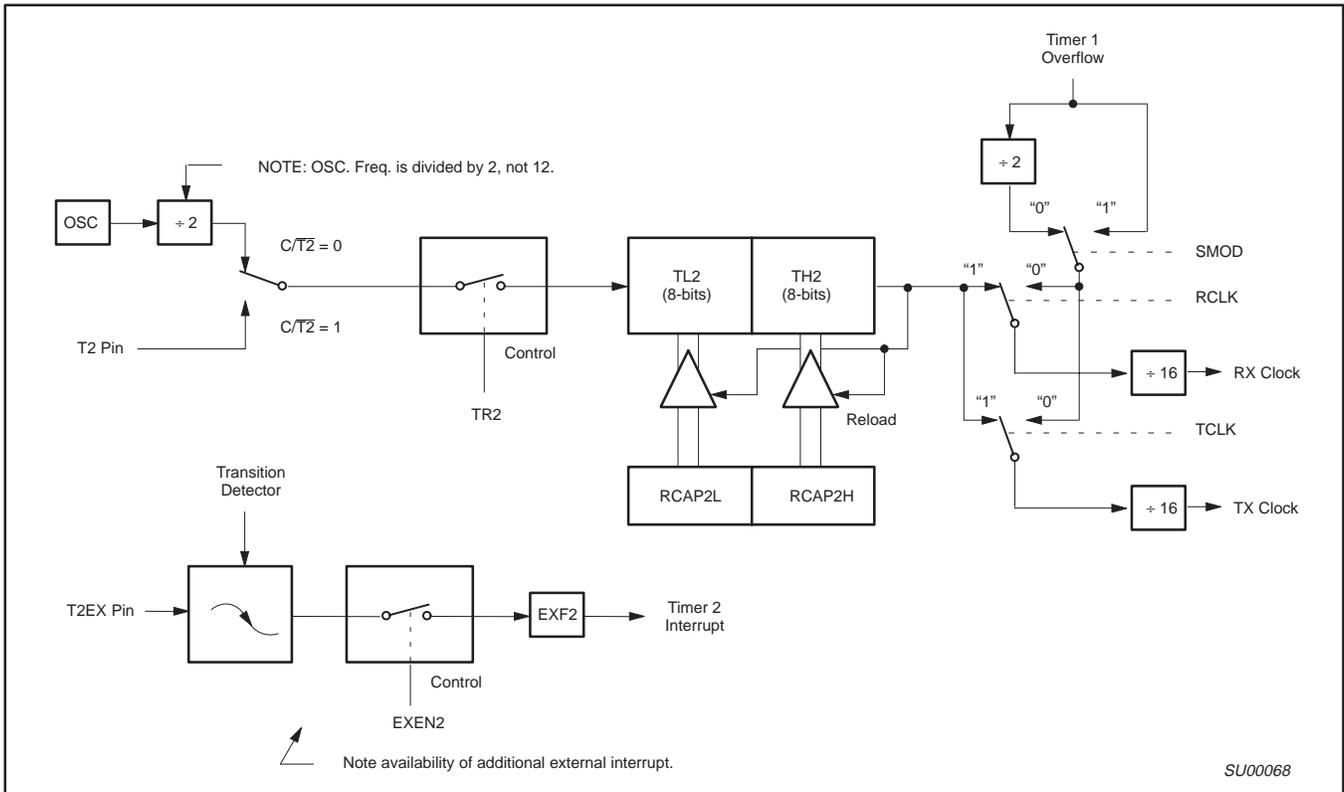
Figure 4. Timer 2 in Baud Rate Generator Mode
