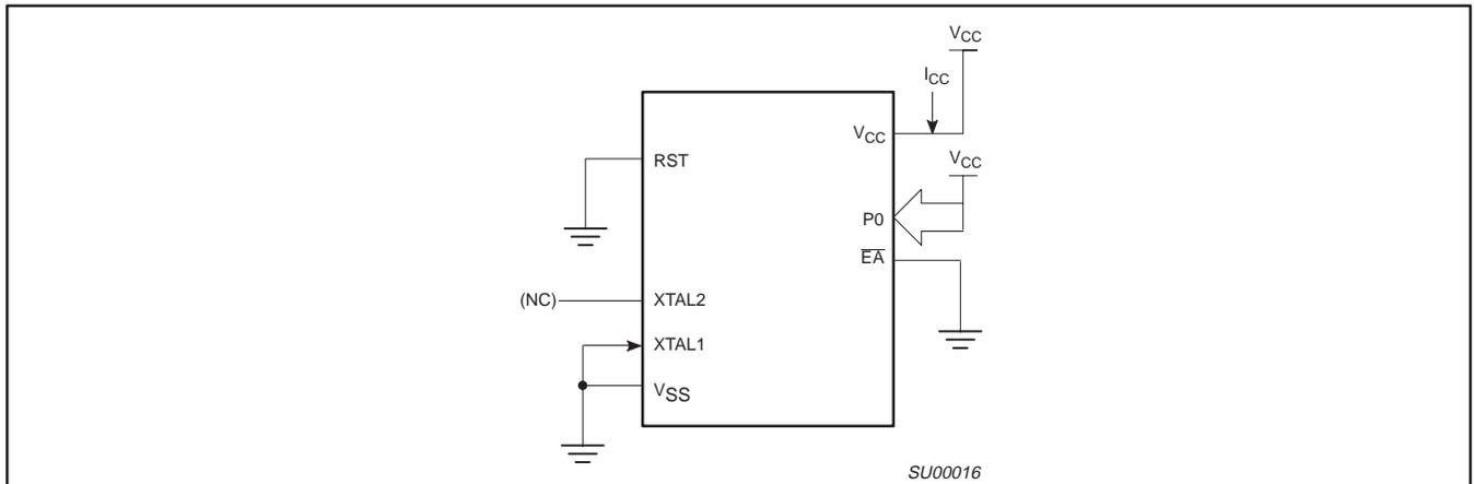
Figure 20.  $I_{CC}$  Test Condition, Power Down Mode
