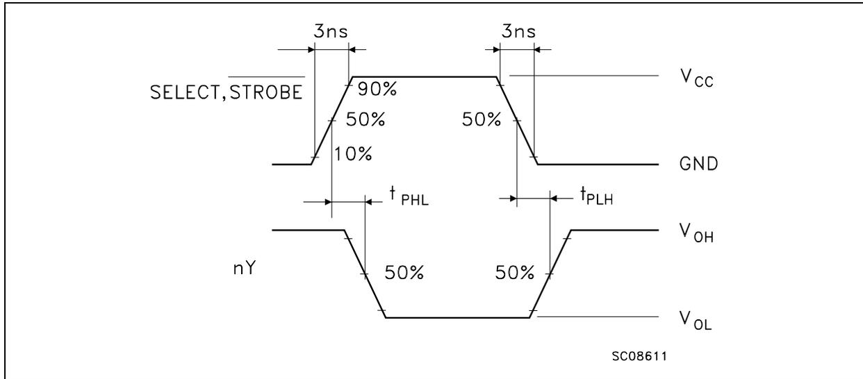
**WAVEFORM 2: PROPAGATION DELAYS FOR NON-INVERTING CONDITIONS**
