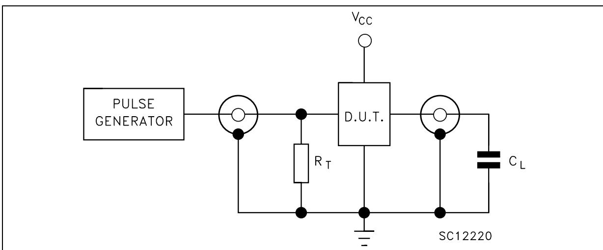
C<sub>L</sub> = 15/50pF or equivalent (includes jig and probe capacitance)
