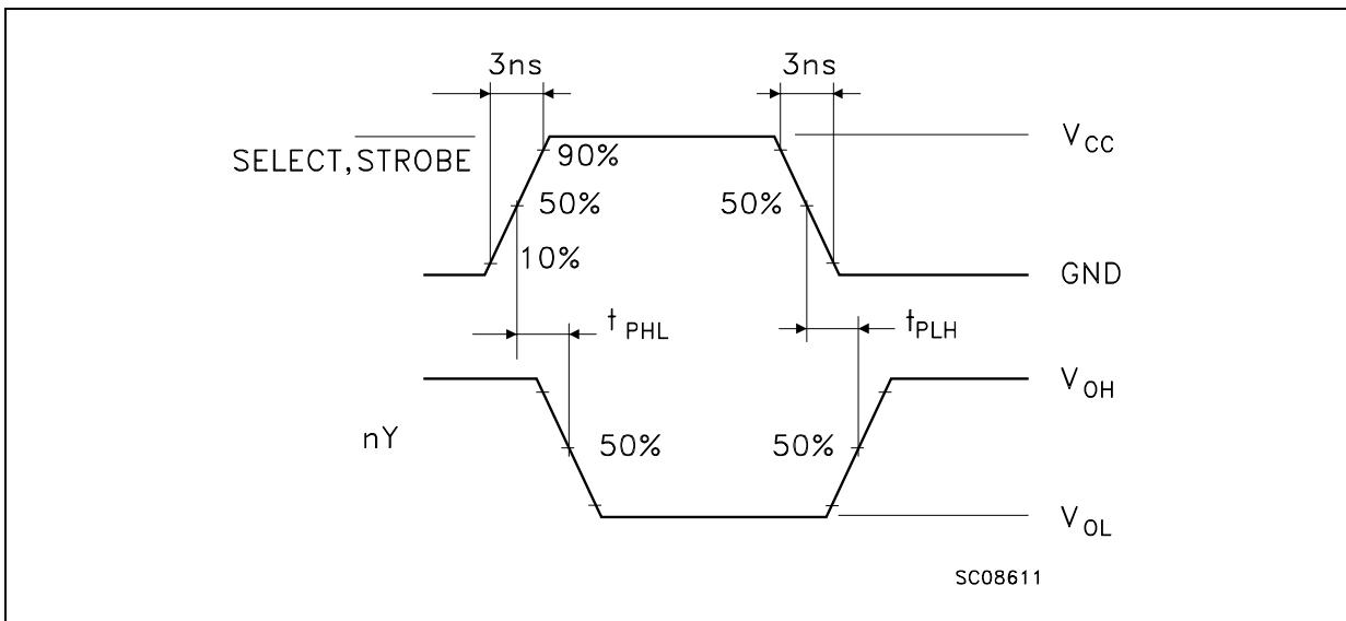
**WAVEFORM 2 : PROPAGATION DELAYS FOR NON-INVERTING CONDITIONS**
