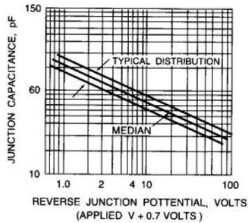
NOTE: WHEN PLOTTING CAPACITANCE VERSUS VOLTAGE IT IS CONVENIENT TO PLOT ON LOG-LOG PAPER AND TO PLOT APPLIED VOLTAGE PLUS BARRIER POTENTIAL (BARRIER POTENTIAL - 0.7 VOLTS) AS THE ABSCISSA. THIS WILL GIVE A STRAIGHT LINE OF SLOPE APPROXIMATELY 1/2 OF WHICH CAN BE EASILY EXTRAPOLATED. CAPACITANCE AT ZERO APPLIED VOLTS IS FOUND AT 0.7 VOLTS ON THE PLOT. THIS TECHNIQUE WAS USED FOR THE CURVE SHOWN.
