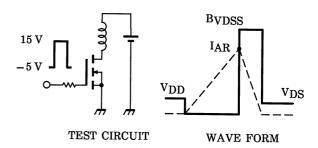
$$\begin{aligned} R_G &= 25~\Omega \\ V_{DD} &= 25~V,~L = 236~\mu H \end{aligned} \qquad E_{AS} &= \frac{1}{2} \cdot L \cdot I^2 \cdot \left( \frac{BVDSS}{BVDSS - V_{DD}} \right) \end{aligned}$$
