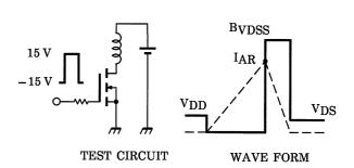
$$\begin{aligned} &RG = 25~\Omega \\ &V_{DD} = 90~V,~L = 7.01~mH \end{aligned} \qquad E_{AS} = \frac{1}{2} \cdot L \cdot I^2 \cdot \left( \frac{BV_{DSS}}{BV_{DSS} - V_{DD}} \right)$$
