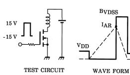
$$\begin{aligned} &RG = 25~\Omega \\ &V_{DD} = 90~V,~L = 48.4~mH \end{aligned} \qquad E_{AS} = \frac{1}{2} \cdot L \cdot I^2 \cdot \left( \frac{B_{VDSS}}{B_{VDSS} - V_{DD}} \right)$$
