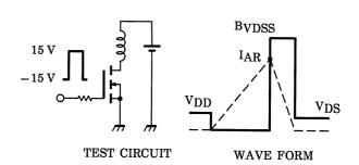
$$\begin{aligned} R_G &= 25 \ \Omega \\ V_{DD} &= 25 \ V, \ L = 272 \ \mu H \end{aligned} \qquad EAS = \frac{1}{2} \cdot L \cdot I^2 \cdot \left( \frac{BVDSS}{BVDSS - V_{DD}} \right) \end{aligned}$$
