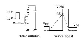
$$\begin{aligned} &R_G = 25~\Omega \\ &V_{DD} = 25~V,~L = 11.6~mH \end{aligned} \quad EAS = \frac{1}{2} \cdot L \cdot I^2 \cdot \left( \frac{BVDSS}{BVDSS - VDD} \right)$$
