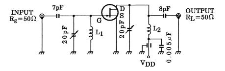
$L_1{:}~0.8~\text{mm}\phi~\text{A}_g$  plated Cu wire 3 turns, 10 mm ID, 10 mm length
