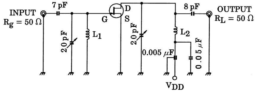
L1: 0.8 mmφ Ag plated Cu wire 3 turns, 10 mm ID, 10 mm length
