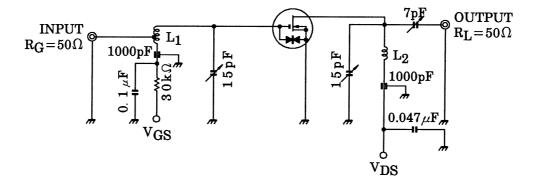
$L_1$ : 1.0 mm $_{\varphi}$  silver plated copper wire 4.0 T, 8 mm $_{\varphi}$  ID TAP at 1.0 T from coil end
