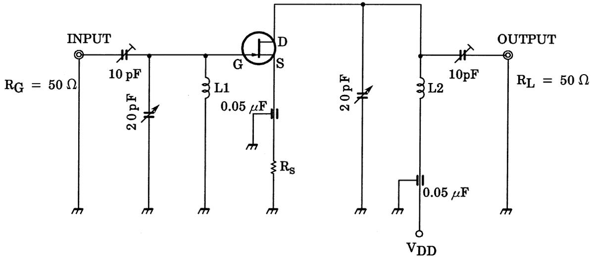
L<sub>1</sub>: 0.8 mmφ A<sub>g</sub> plated Cu wire, 3 turns, 10 mm ID, 10 mm length.
