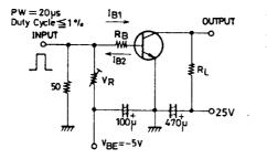
I C=10 I B1=-10 I B2=500mA, V CC=25V (For PNP, the polarity is reversed.)
