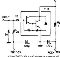
$$\label{eq:pwp} \begin{split} &(For\ PNP,\ the\ polarity\ is\ reversed.)\\ &PW = 50\mu s,\ Duty\ Cycle \leqq 1\%\\ &500I_B1 = -500I_B2 = I_C = 5A\\ &Unit\ (resistance:\Omega, capacitance:F) \end{split}$$
