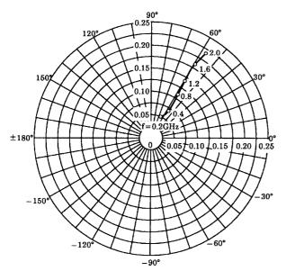
$S_{22e}$   $V_{CE} = 5V$   $I_{C} = 5mA$   $T_{a} = 25^{\circ}C$ (UNIT : O)
