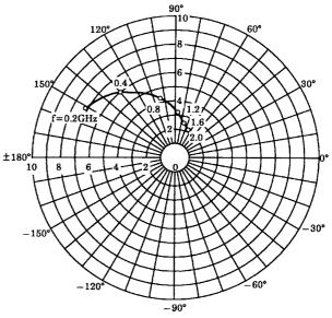
$\begin{array}{l} S_{12e} \\ V_{CE} = 6V \\ I_{C} = 7mA \\ Ta = 25^{\circ}C \end{array}$
