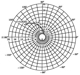
$S_{12e}$   $V_{CE}=8V$   $I_{C}=5mA$   $T_{a}=25^{\circ}C$
