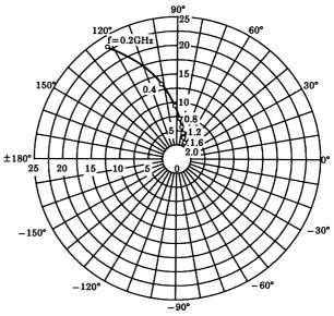
$\begin{array}{l} S_{12e} \\ V_{CE} = 8V \\ I_{C} = 20 mA \\ Ta = 25 ^{\circ}C \end{array}$
