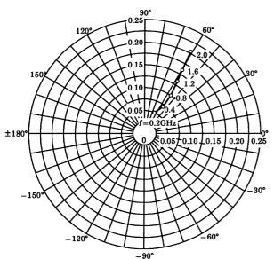
$S_{22e}$   $V_{CE}=8V$   $I_{C}=5mA$   $T_{a}=25^{\circ}C$   $(UNIT: \Omega)$
