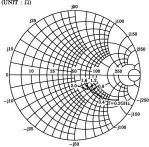
$\begin{array}{l} S_{11e} \\ V_{CE} = 8V \\ I_{C} = 20 mA \\ T_{a} = 25 ^{\circ}C \\ (UNIT:\Omega) \end{array}$
