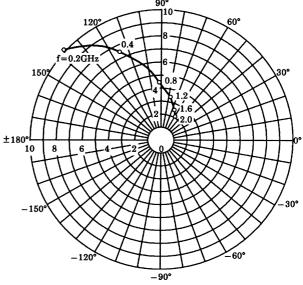
$S_{12e}$   $V_{CE}=8V$   $I_{C}=5mA$   $T_{a}=25^{\circ}C$
