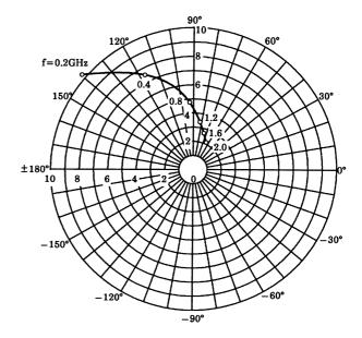
$\begin{array}{c} S_{12e} \\ V_{CE} = 5V \\ I_{C} = 5mA \\ Ta = 25^{\circ}C \end{array}$
