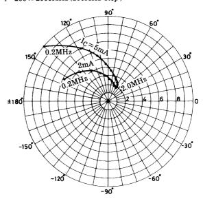
$\begin{array}{l} S12e:V_{CE}\!=\!5V\\ f\!=\!200\text{ to }2000M\text{Hz} \,(200M\text{Hz step}\,) \end{array}$
