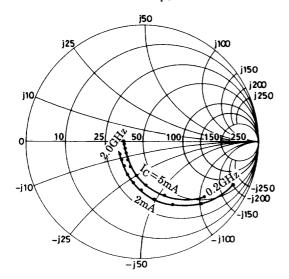
$S21e:V_{CE}\!=\!5V$   $f\!=\!200$  to 2000MHz (200MHz step )
