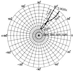
$S22e:V_{CE}\!=\!5V\\f\!=\!200$  to 2000MHz (200MHz step )
