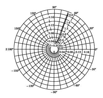
$\begin{array}{l} S_{22e} \\ V_{CE} = 6V \\ I_{C} = 7mA \\ Ta = 25^{\circ}C \\ (UNIT:\Omega) \end{array}$
