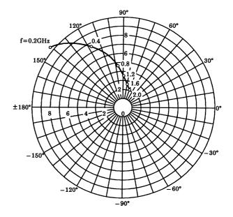
$S_{12e}$   $V_{CE}=8V$   $I_{C}=5mA$   $Ta=25^{\circ}C$
