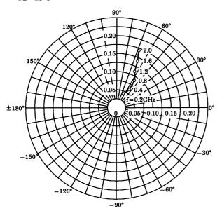
$\begin{array}{l} S_{22e} \\ V_{CE} = 8V \\ I_{C} = 20 mA \\ T_{a} = 25 ^{\circ}C \\ (UNIT:\Omega) \end{array}$
