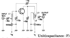
$L_1$ : 1mm $\phi$  plated wire, 10mm $\phi$  5T, pitch 15mm,
