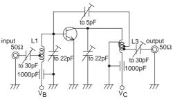
$L1:1mm\varphi \ plated \ wire, \ 10mm\varphi \ 5T, \ pitch \ 15mm, \\ tap:2T \ from \ base \ side$
