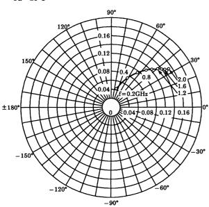
$S_{22e}$   $V_{CE} = 6V$   $I_{C} = 3mA$   $Ta = 25^{\circ}C$   $(UNIT : \Omega)$
