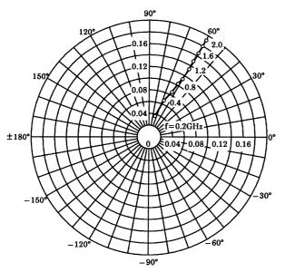
$\begin{array}{c} S22e \\ VCE = 6V \\ IC = 3mA \\ Ta = 25^{\circ}C \\ (UNIT:\Omega) \end{array}$
