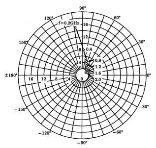
$\begin{array}{l} S_{22e} \\ V_{CE} = 10V \\ I_{C} = 40 \text{mA} \\ T_{a} = 25 ^{\circ}\text{C} \\ (U\text{NIT}: \Omega) \end{array}$
