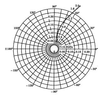
$\begin{array}{l} S_{21e} \\ V_{CE} \! = \! 10V \\ I_{C} \! = \! 20 mA \\ Ta \! = \! 25 ^{\circ}\! C \end{array}$
