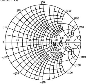
$\begin{array}{l} S_{11e} \\ V_{CE} = 10V \\ I_{C} = 40 mA \\ Ta = 25 ^{\circ}C \\ (UNIT: \Omega) \end{array}$
