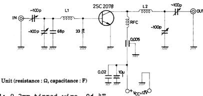
Coil data L1: 0.3mm tinned wire, 9ø 4T
