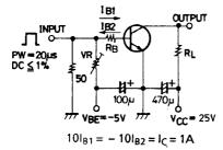
(For PNP, the polarity is reversed.) Unit (resistance :  $\Omega$ , capacitance : F)
