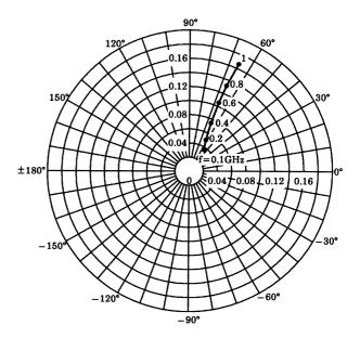
$S_{21e}$   $V_{CE} = -5V$   $I_{C} = -10\text{mA}$   $Ta = 25^{\circ}C$
